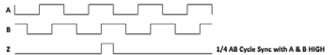
Standard Phasing: A Leads B for CW Rotation (viewed from back of encoder)
